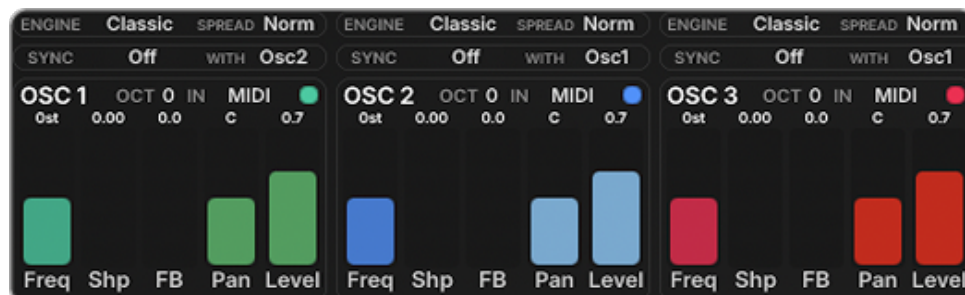
Figure 3: Oscillators 1, 2 and 3 — multi-engine layout. Each oscillator shows 5 faders (Freq, Shape, FB, Pan, Level) below the engine selector and source dropdown.
