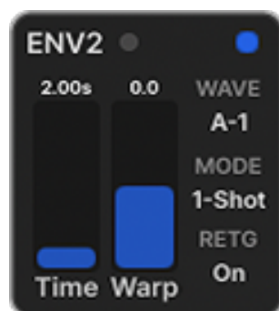
Figure 15: Envelope 2 — vector envelope module with time, warp and shape selection. Wavetable-based envelope with 100 predefined shapes (10 banks × 10 shapes).
