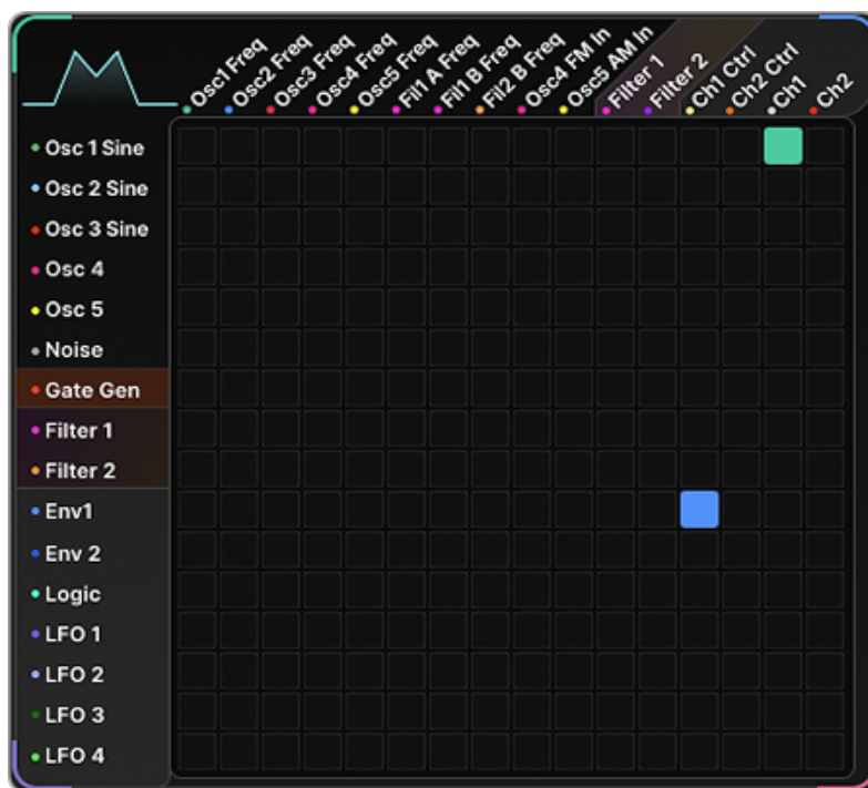
Figure 29: Modulation Matrix — 16x16 grid. Rows are modulation sources (Osc 1-5, Noise, Gate Gen, Filters, Envs, LFOs, Logic). Columns are destinations (any modulatable parameter via right-click, plus fixed audio routes for filter/channel I/O).
