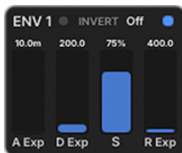
Figure 14: Envelope 1 — classic ADSR with attack, decay, sustain and release stages plus invert toggle. Traditional 4-stage envelope with selectable curve types and output inversion.
