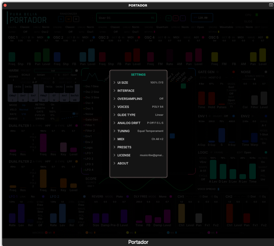
Figure 32: Settings panel — UI size, interface, oversampling, voices, glide, tuning, analog drift, MIDI and presets configuration.
