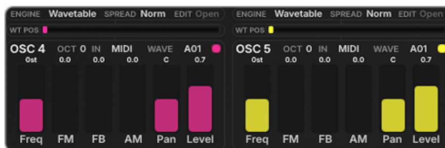
Figure 4: Oscillators 4 and 5 — wavetable multi-engine layout. Each shows 6 faders (Freq, FM/PM, FB or engine-specific, AM/RM, Pan, Level) plus the Wave selector and engine slot.
